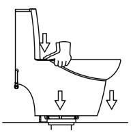
5. Place the bolt cap bases on the T-bolts and proceed to secure the toilet into place by fastening the washers and nuts to the bolt caps and T-bolts.
