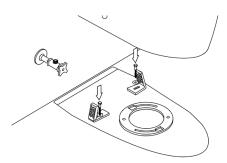
4. Turn toilet on its side (please protect the ground surface with soft material to prevent damage to toilet), and press new wax seal firmly around waste flange. apply a small bead of silicone sealant around toilet base.
