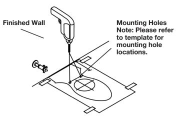
\*\*NOTE: For floors less than 1-1/2" (38 mm) thick use a 5/32" bit. For floor thicker than 1-1/2" (38 mm) use a 3/8" bit for anchor (required) installation.\*\*
